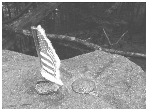
Benchmark on top of Mount Rogers (Elev. 5,729 feet). Note USGS carved into rock face.
