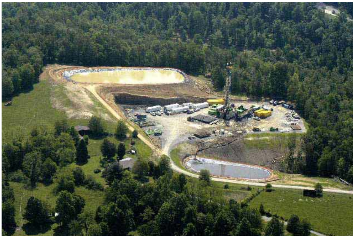
Well site during active drilling to the Marcellus Shale formation in Upshur County, West Virginia, in 2008. (An additional water storage pit is not in the photo.) Copyright WVSORO.
