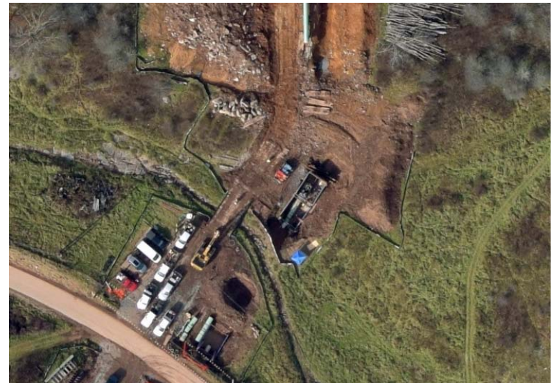
ATLANTIC COAST PIPELINE STREAM CROSSING IN POCAHONTAS COUNTY. THE CROSSING DOES NOT CONFORM TO THE METHOD SPECIFIED IN APPROVED PLANS.
